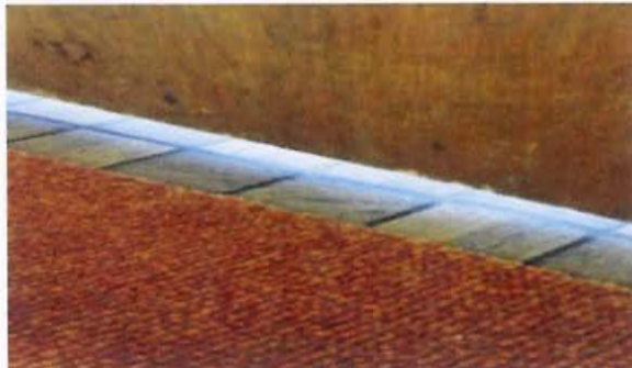
Material: Linoleum and Mastic - Wood Squares HMR #: 29 Asb: Comment:
